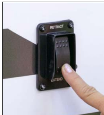
Power switch for PSX 2025012486 and 2025049967
