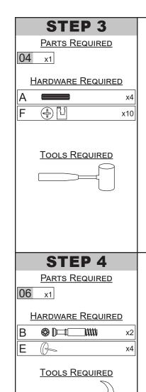
IMPORTANT: Install Tack Glides (E) before installing Cam Screws (B).
