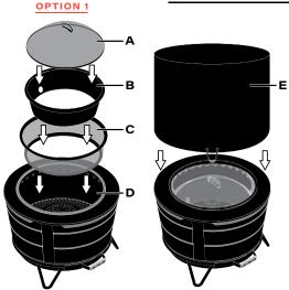
When the Fire Pit is not in use, you may nest the accessories inside Fire Pit. First, invert the lower screen (C) and place it inside the Fire Pit (D). Next, put the heat deflector (B) right-side up in the inverted lower screen (C). Place the upper screen (A) on top. Finally, place the cover (E) (included with the Fire Pit purchase), over the top.
