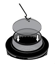
After a Wood Pack or firewood has been added, place the top piece back on with the poker. Ensure that it is securely nested.
