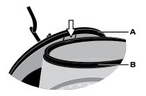
To add an additional Wood Pack or firewood, remove the top piece (A) of the screen with the included poker (see page 6 for assembly), and gently hang on the side of the bottom piece (B).
