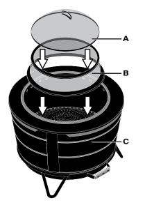
Place both top (A) and bottom (B) pieces of the screen on the top ring of the Fire Pit (C). Ensure that they are securley nested.
