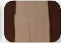
Panel C SM-1 Degreaser Dilution Rate 1:40 Scrub Test Cycles: 75
