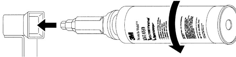
2. Inspect threads on main nozzle. **Periodic use of lithium grease or petroleum jelly on the threads is recommended.** If threads become damaged, replace with new main nozzle.
