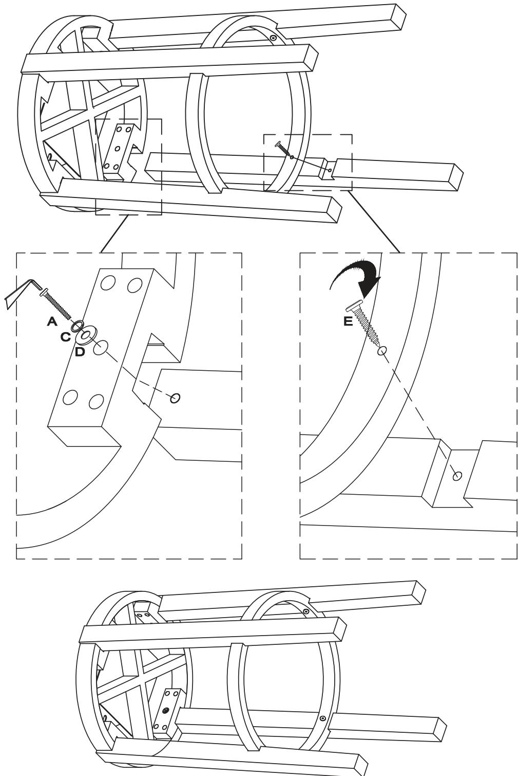
Do not tighten bolts completely until all bolts are completely lined up and inserted into holes.
