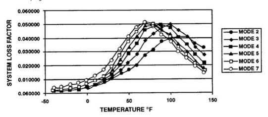
**Test Method:**The following data were obtained by doing a frequency sweep from 1 to 100 radians/sec (0.16 to 16 Hz) at 5 different temperatures:  $-20^{\circ}$ ,  $10^{\circ}$ ,  $0^{\circ}$ ,  $10^{\circ}$ , and  $22^{\circ}$ C. A 3 point bend geometry was used on the Rheometics RSA II. Time – temperature superposition was used to create the master curve for a reference temperature of  $22^{\circ}$ C.
