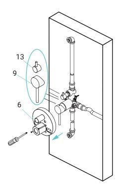
• If finishing on tiled wall, remove the handle (9) and diverter (13) and put the cover plate (6) back over the valve. Remove cover plate after finished wall is complete.
