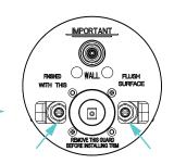
The valve body is with water flow regulation function. If there is great deviation in cold and hot water flow, it could be adjusted at the point indicated by the arrow. (Turn down in clockwise rotation)
