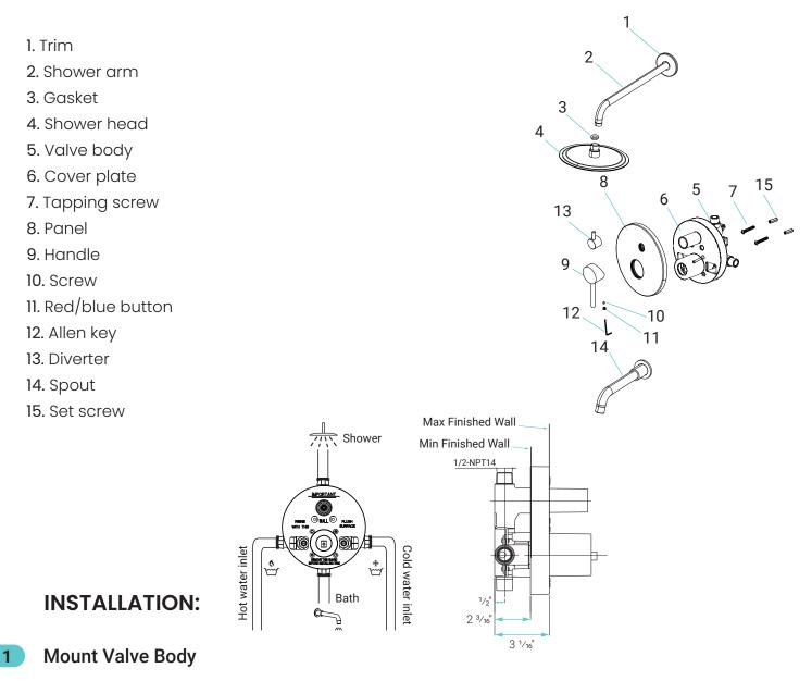
• Following the installation reference size, insert two set screws (15) for the valve body mounting.
