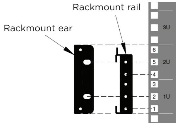
Position the guide screw on the back of the rackmount rails into the rear rack square holes to temporarily support the rails in place.
