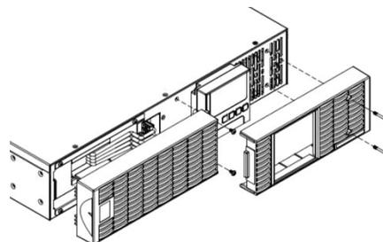
**Step 5:** Install the front panels. Execute a battery test via the LCD control panel, go to the Configuration Menu, then scroll to the UPS Diagnostic then select battery test and Activate, then scroll to ResetReplaceBAT to reset the battery replacement date. This operation can also be done via PowerPanel® Business Edition Agent or RMCARD web interface. Please see their respective User Manuals for detailed instructions.
