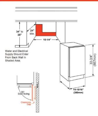
When installing with the hinge side next to a wall, leave adequate space for your door handle.
