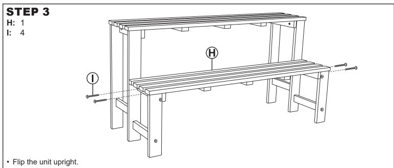
• Place Bottom Shelf (H) onto the lower level of the stand and secure it using four M6x45 Bolts (I).
