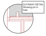
TO ACCOMMODATE THE HINGE PINS ON THE HINGE SIDE OF THE PANEL Drill a hole at least 5/16" in diameter and 1" deep into the top and bottom of the frame in the location shown.
