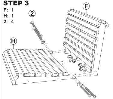
Loosely fasten Backrest (F) to Seat (H) using four M10x65mm Bolt Sets (2).
