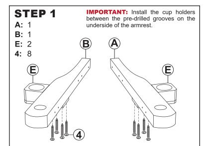
Align one Cup Holder (E) with Right Armrest (B) and secure using four M4x30mm Screws (4).
