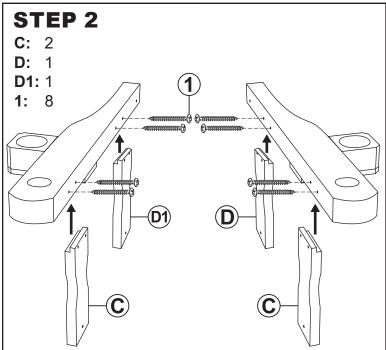
Secure one Front Arm Support (C) and Right Back Armrest Support (D1) to the right armrest using four M4x40mm Screws (1).
