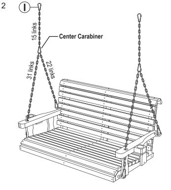
Link the carabiner on the second-longest chain to arm eye bolt. Link the the longest chain to the eye bolt on the front of the seat. Disconnect the longest chain from the center carabiner, run the chain up through the bottom of the hole in the armrest, reconnect it to the center carabiner.
