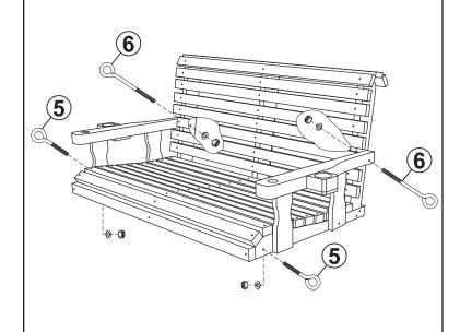
Secure the back of the armrests to the seat using two Arm Eye Bolt Sets (6), as shown.
