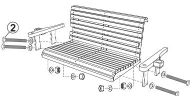
Loosely secure the armrest supports to the seat using four M10x65mm Bolt Sets (2).
