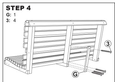
Loosely secure Back Brace (G) to the backrest and loosely se, as shown.
