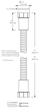
Specifications: Inlet / Outlet: 1/2"-14 NPSM Threaded Swivel Connector
