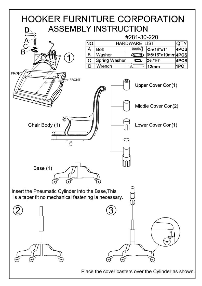
Place the chair body onto the cylinder. No mechanical fastening is necessary because this is a taper fit. Now sit in the chair. This will firmly secure the taper fit.
