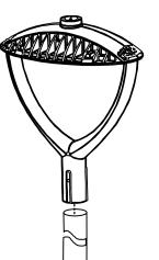
8 Install the included shunt to the top of the fixture by aligning the prongs. Turn clockwise to lock in. If photocell (*sold seperately*) is desired, remove shunt and install as per shunt installation.
