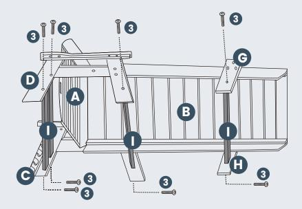
Position the supporting pole into the brackets on the rear legs for a comfortable rest.
