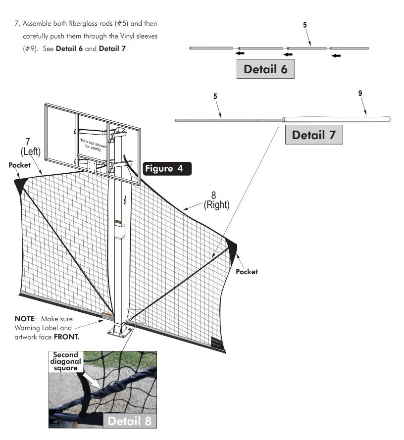
8. As shown, insert one end of the fiberglass rod into the triangular pocket on the FRONT upper outside corners of the net. The rod will then remain on the front of the net until it reaches the **second** diagonal square from the lower inside corner as shown in **Detail 8**. Please push it though this hole and down into the fiberglass rod pivot connector. Then carefully take the fiberglass tube sleeve and slide it over the pivot connector as well. Do this for both sides.
