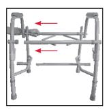
Repeat steps 1 and 2 to attach the Bucket Frame and Frame Support Bar to the other Armrest Assembly.
