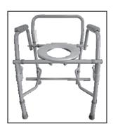
5. Align the Toilet Seat to the opening in the Bucket Frame and the Toilet Seat clamps to the back rail of the Bucket Frame. Push down on Toilet Seat until clamps snap firmly into place. Repeat for the lid.
