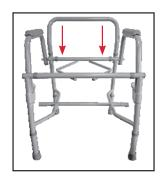
4. Attach the Backrest to the Backrest Receptacles in the Armrest Assembly by depressing the brass push button on the Backrest and sliding it into the corresponding hole in the Backrest receptacles. Ensure the push button is fully engaged through the hole.
