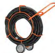
CF Cable Feeding Tool (Standard with Model 88) Helps work cable around tight bends.
