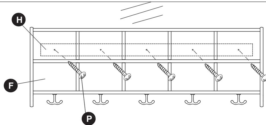
Two adults recommended to attach the shelf to (H) by 5 screws (P) via holes on the back of panel (F). ((H) is attached to wall in the previous step)
