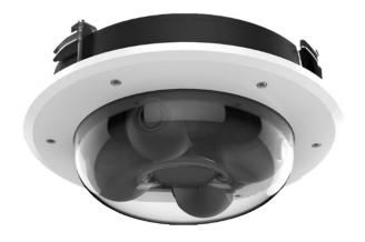
Hikvision's DS-2CD6D54G1-ZS/RC PanoVu Flexible Outdoor Network Camera features 1/2.7" progressive scan CMOS sensors and four lenses. Each lens supports a resolution of up to 2560 x 1920 at 24 fps. Compression up to H.265+ saves bandwidth and storage space.
