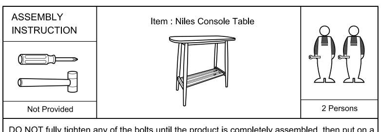
DO NOT fully tighten any of the bolts until the product is completely assembled, then put on a a flat surface to make sure the product is level and then fully tighten all the bolts.
