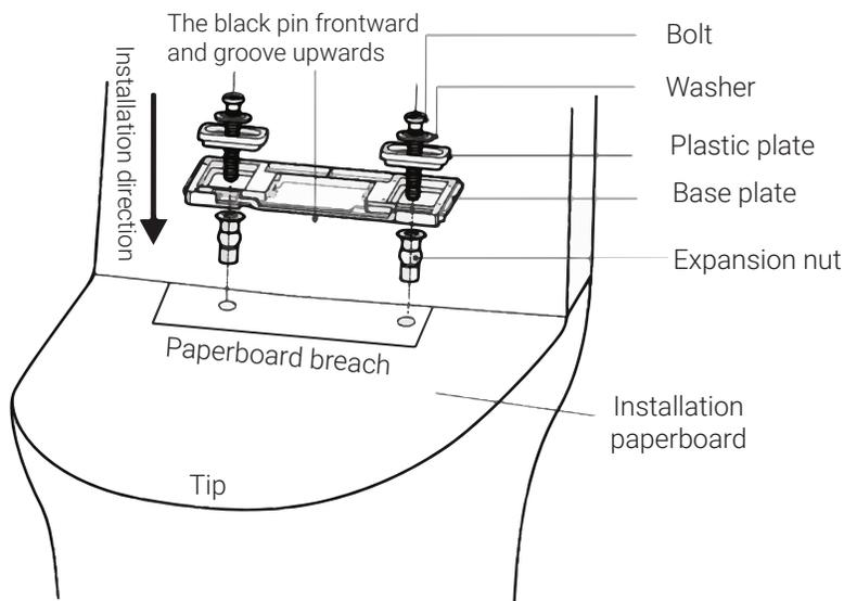
**NOTE:** Unfold the installation paperboard, align the paperboard to fit the ceramic bowl from the tip, then insert the base plate to the paperboard breach to make sure the base plate aligns with the paperboard breach.
