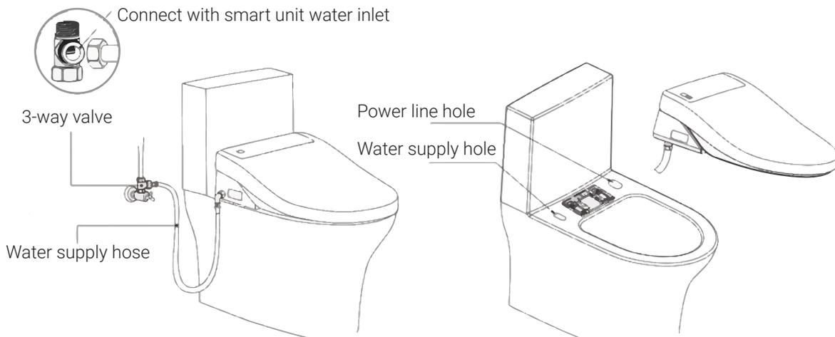
**NOTE:** Do not distort or damage the supply hose to avoid any leakage. Do not use water supply hose and other accessories of other brands, which may cause danger. Do not recommend to use old water supply hose and accessories, which may cause danger.
