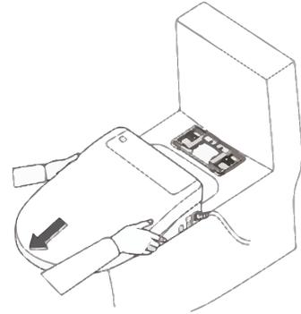
**NOTE:** Before pulling out the washlet, release hand from "removal button".
