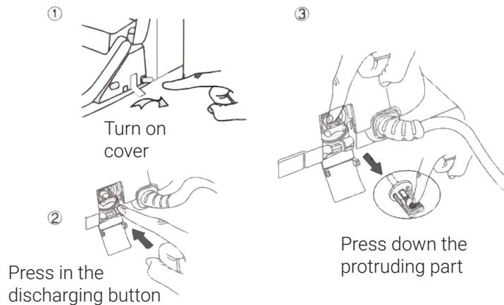
**⚠ WARNING:** Before water starts discharging, the power must be turned off!
