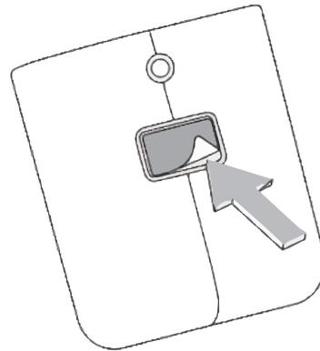
3. Insert wall anchor into the hole in the wall. Install the hanger to the wall with a screw and stick the double-faced adhesive tape to the wall and tighten the screw.
