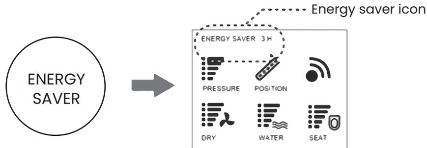
2. Press “ENERGY SAVER” button again, LCD screen shows figure 6, and the “ENERGY SAVER” icon will disappear after 3 seconds. The toilet enters the energy saver mode from 9:00 to 15:00 every day. During this period, the power light is off, and the energy saver light is on. It goes back to normal operation mode after the energy saver time.
