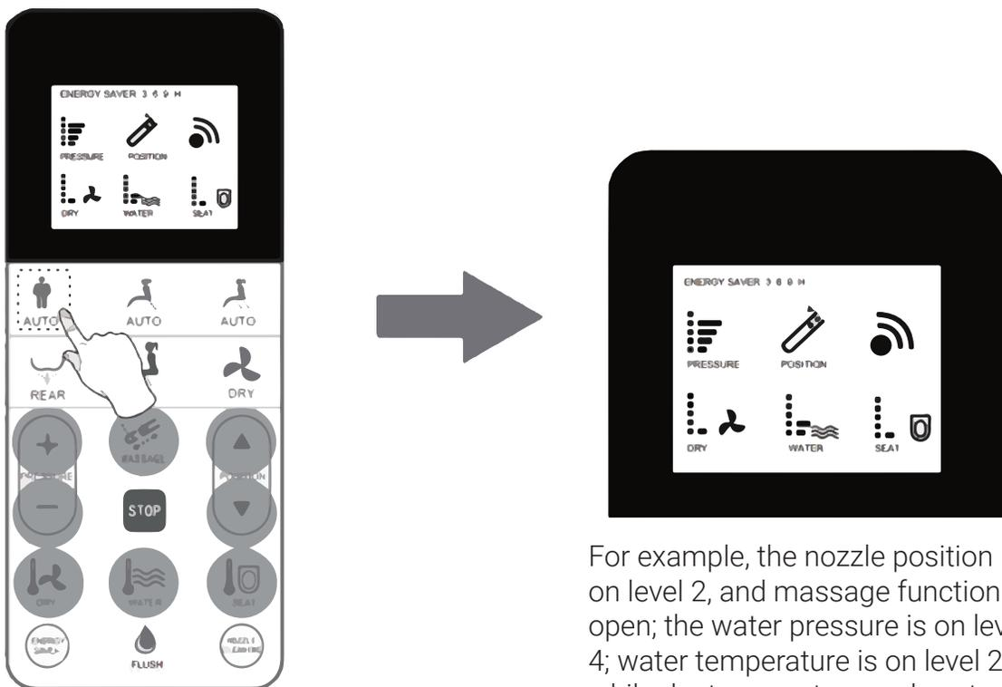
For example, the nozzle position is on level 2, and message function is open; the water pressure is on level 4; water temperature is on level 2, while dry temperature and seat temperature are on level 1.
