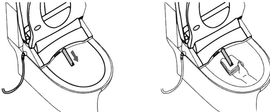
**NOTE:** Do not apply force when pushing or pulling the wand, as this may damage the mechanism.
