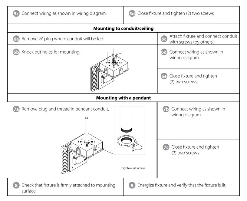
**IMPORTANT:** To weather-proof your outdoor installation, be sure to seal all mounting points, wire inlets, and penetrations (Conduit, Plugs, etc.) with silicone sealant.
