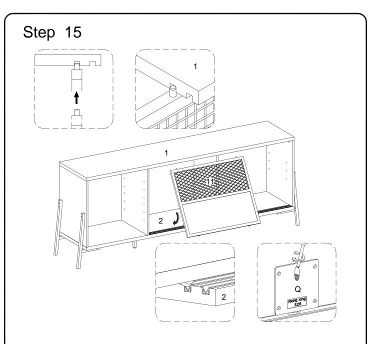
Insert the upper pins of part (11) into the groove of part(1).Lift up the door in vertical position with the bottom panel (2) ,lay down the door and keep the wheels matching with the track in bottom panel as per diagram .
