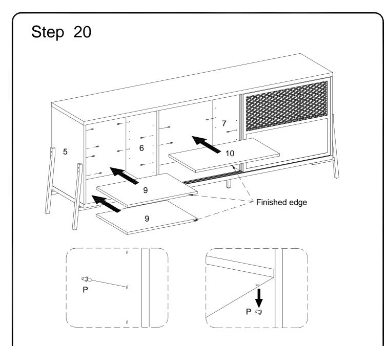
Insert shelf support pin (P) into parts (5,6,7) as per diagram. Make sure you place the shelf support pins (P) in the same level. So the shelf is not titled .Put parts (9,10) into unit as per diagram. Tilt and rest the adjustable shelves (9,10) onto the shelf support pins .
