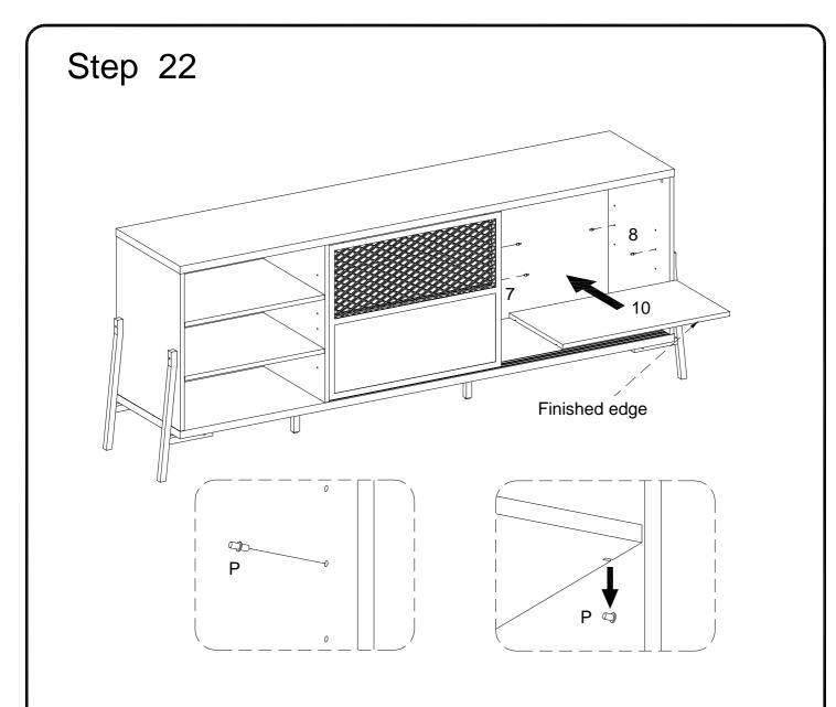
Insert shelf support pin (P) into parts (7,8) as per diagram. Make sure you place the shelf support pins (P) in the same level. So the shelf is not titled .Put part (10) into unit as per diagram. Tilt and rest the adjustable shelf (10) onto the shelf support pins .
