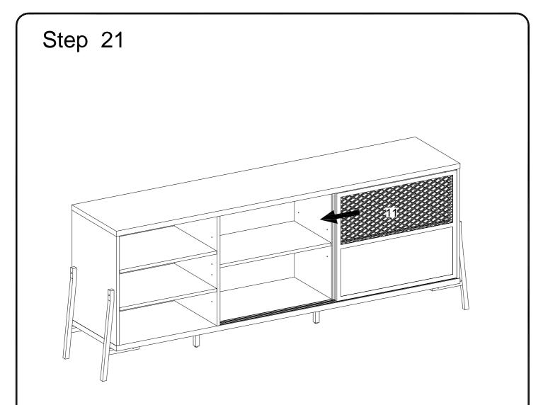
Slide the doors (11) to the left and right as per diagram.
