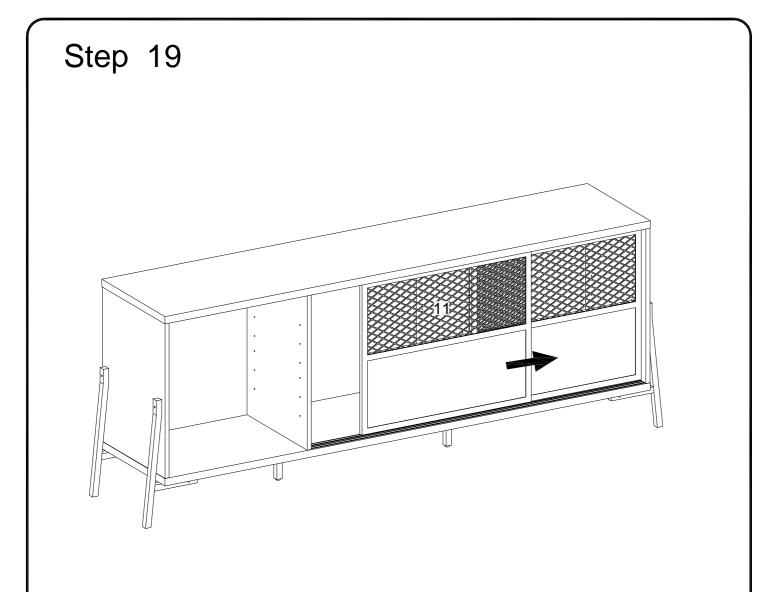
Slide the doors (11) to the left and right .If necessary , re-assemble the doors for a good fit and sliding smoothly.
