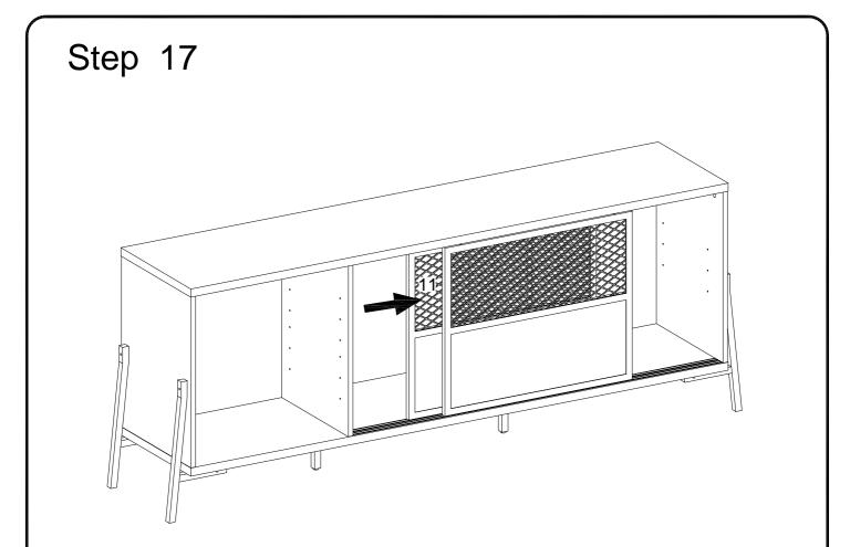
Slide the doors (11) to the left and right .If necessary , re-assemble the doors for a good fit and sliding smoothly.
