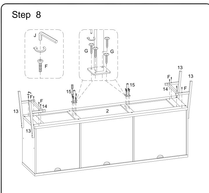
Using bolt (F) attach part (13) to part (2) with Hex key (J) ,then using screw (G) attach part (15) to part (2) with Philips head screwdriver as per diagram.
