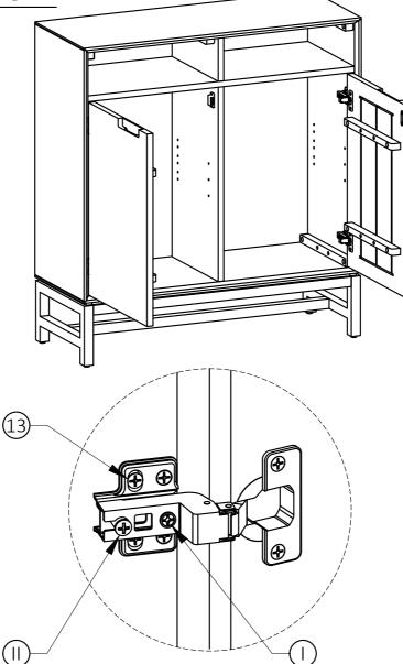
Tighten the Screw marked (I) to fasten hinge. The door may need to be adjusted so that all the spaces between the door and the unit sides are equal. To adjust, follow instructions:
