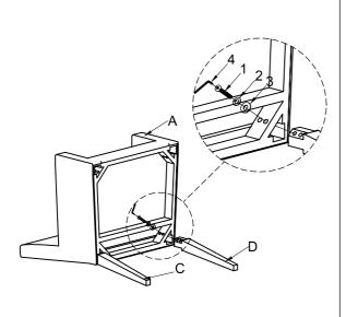
DO NOT TIGHTEN BOLTS COMPLETELY
