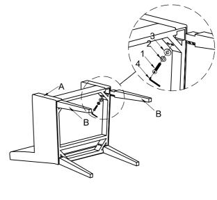
DO NOT TIGHTEN BOLTS COMPLETELY
