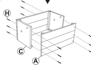
**NOTE:** Each side panel has a ledge for supporting the bottom panel. Ensure the ledge of both side panels is installed on the bottom.
