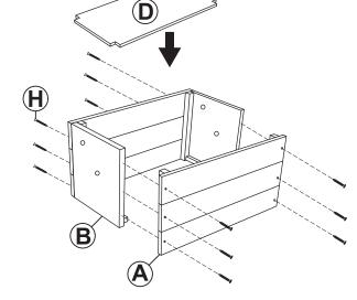
**NOTE:** Each side panel has a ledge for supporting the bottom panel. Ensure the ledge of both side panels is installed on the bottom.
