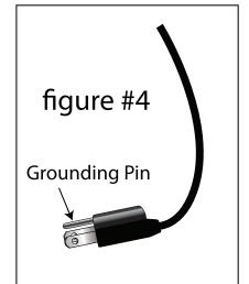
**6. NEVER REMOVE THE GROUND PIN FROM PLUG.** (See figure #4)
