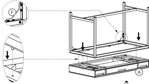
1. Attach the assembled metal frame to Top(A).
