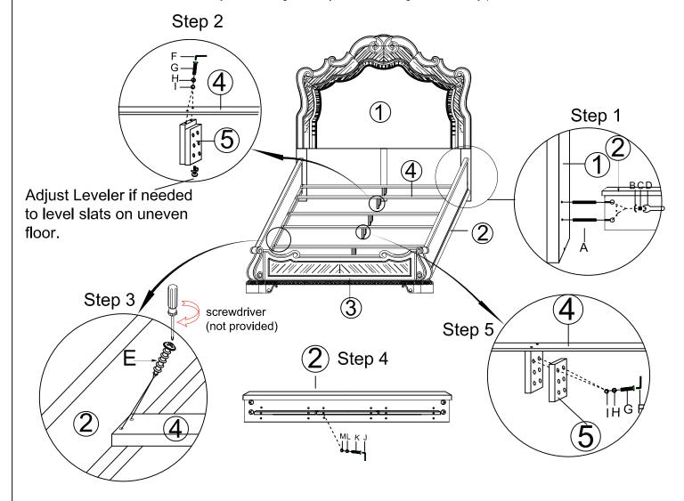
Note 1: You can change the height of slats (4) by adjusting the height of cleat on side rails (2) as shown in step 4.
