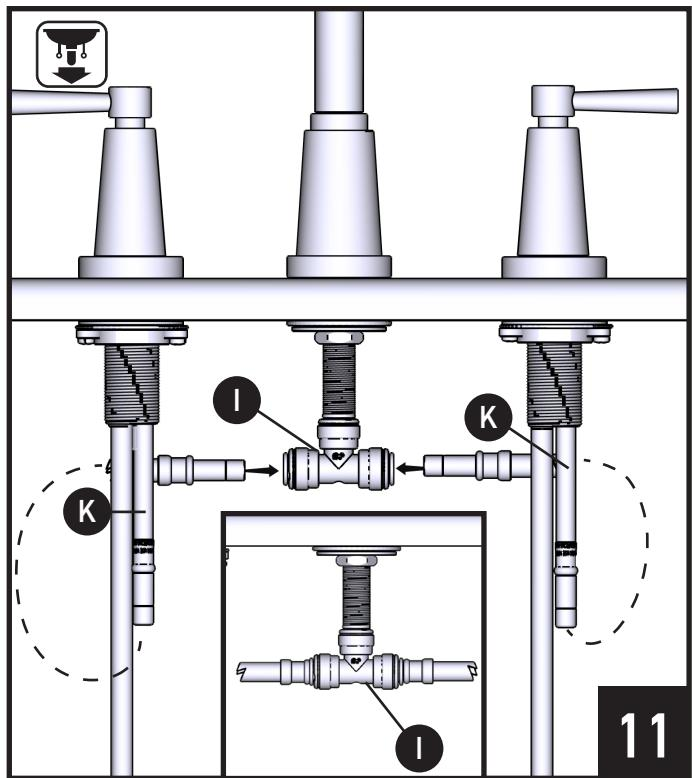
1. Connect Widespread Hose (K) from valve bodies into Tee (I) as shown. Push in as far as possible for full engagement.
