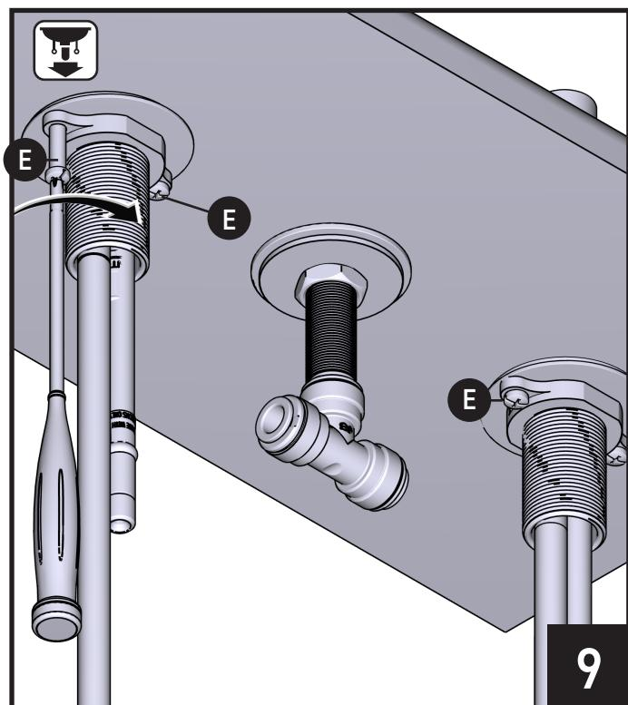
1. Tighten the 4 screws of kit (E) with Phillips screwdriver as illustrated.
