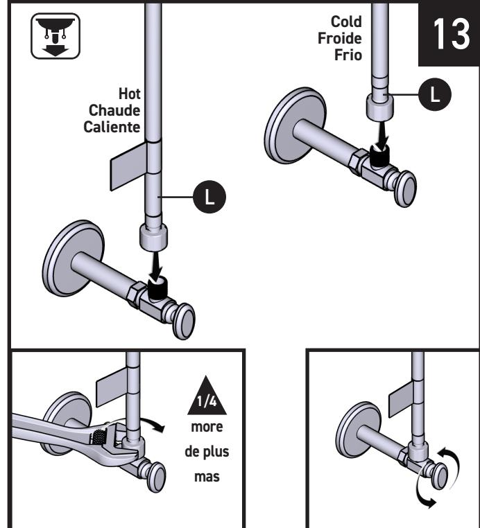
1. Attach hot & cold supply lines (L) to shut off valves. Tighten by hand, then 1/4 turn more with adjustable wrench. Turn on water and check for leaks.
