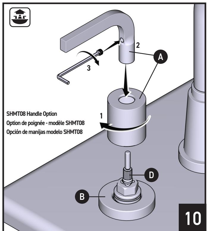
Install Handle Hub Kits (x2) (B), Handles (x2) (A), onto the cartridges (x2) (D). Proceed in numbered order as shown.
