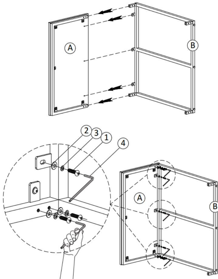
1. Align Side (B) to the openings on each corner of Top (A).
