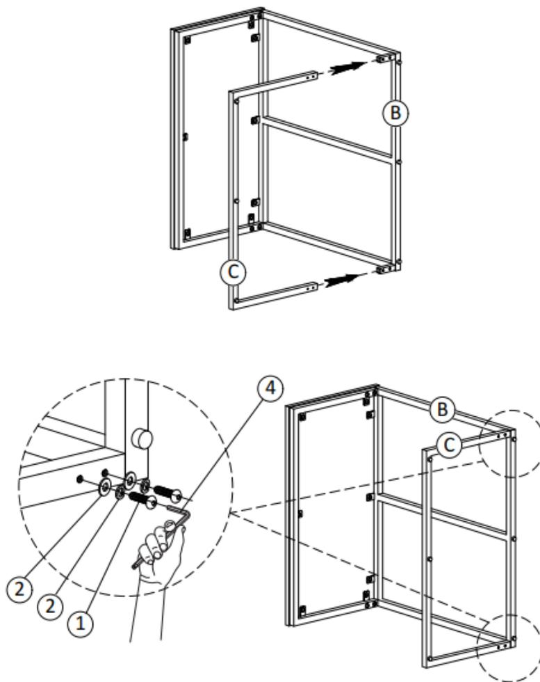
1. Align Base (C) to the openings on each corner of Side (B).
