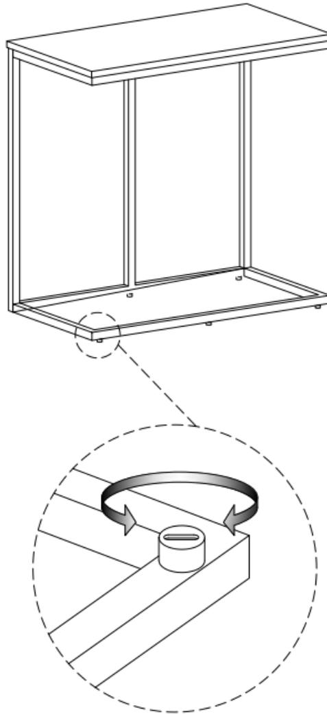
**NOTE:** Levelers on the bottom of the sides can be adjusted if floor is uneven.
