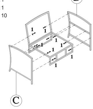
Do not fully tighten hardware until all components in this step have been connected.
