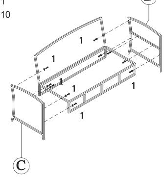
Do not fully tighten hardware until all components in this step have been connected.
