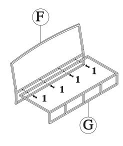
Do not fully tighten hardware until after Step 5 is complete.
