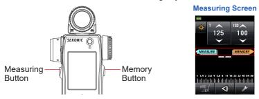
Auto: The button arrangement is set to "Standard" when the incident light system is selected, and to "Reverse" when the reflected light system is selected.
