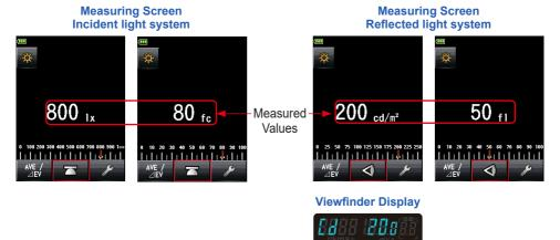
\* If the light receiving method is changed from the incident light system to the reflected light system, the display is automatically changed from the Ambient Light Illuminance (Ix or fc) Mode to the Ambient Light Luminance (cd/m² or fl) Mode.
