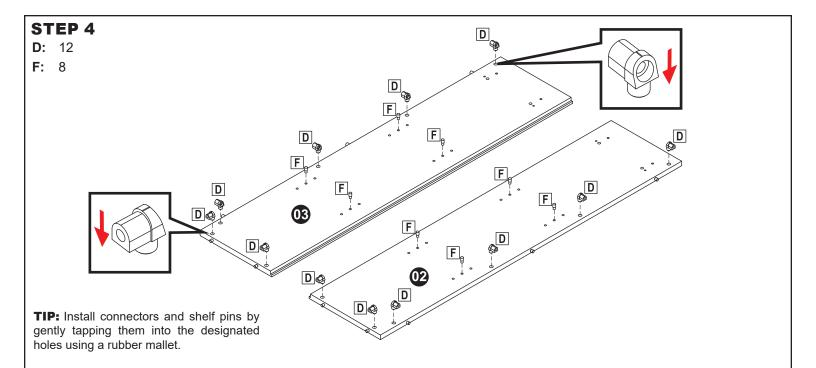
With the angled edges facing the inside of the panel, install six Connectors (D) into Left Side Panel (02) and Right Side Panel (03). Install four Shelf Pins (F) into each side panel as shown in the diagrams.
