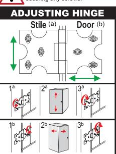
With assistance to hold the door in place, align the hinges of Left Door (15) with the indents on the left stile. Loosely secure each hinge using three M3.5x14mm Pan Screws (L).
