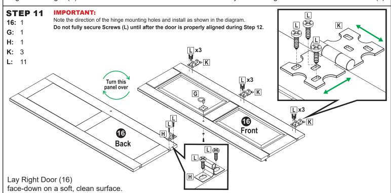
Align Strike (H) with the indents on the bottom of the door and secure using two M3.5x14mm Pan Screws (L). Flip the door over.
