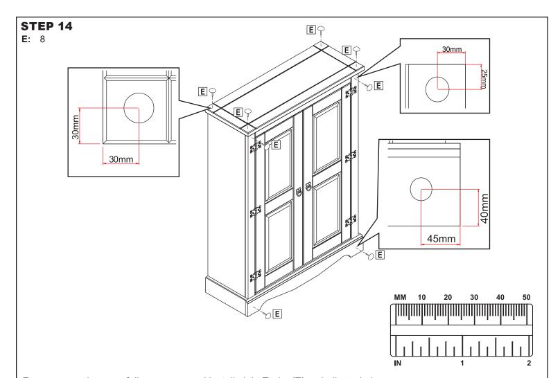
For even spacing, carefully measure and install eight Tacks (E) as indicated above.
