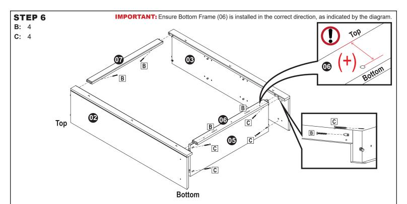
Lay Left Side Panel (02) on a smooth, clean surface. Ensuring the catches face the top of the cabinet, align Bottom Panel (05) just above the bottom connector of the side panel and secure using two M4.5x28mm Pan Screws (C).
