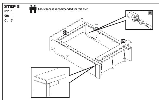
Align Front Trim Board (09) with the bottom, front side of the unit. Have an assistant hold the trim board tightly to ensure it remains flush with the unit while it is secured. From the backside of the bottom frame, secure the trim board using three M4.5x28mm Pan Screws (C).
