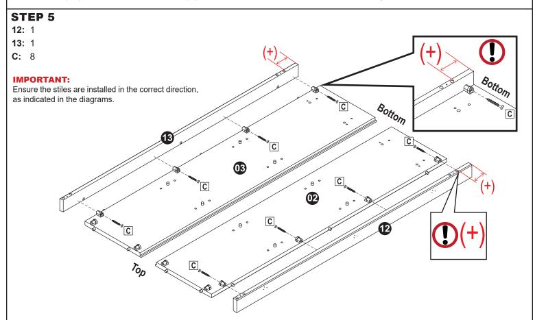
**NOTE:** On the narrow side of the stiles, the 'bottom' has a larger gap between the dowel mounting holes and the end.
