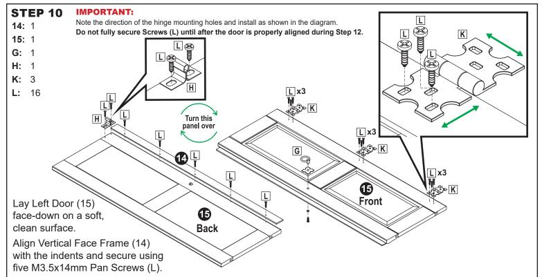
Align Strike (H) with the indents on the bottom of the door and secure using two M3.5x14mm Pan Screws (L). Flip the door over.
