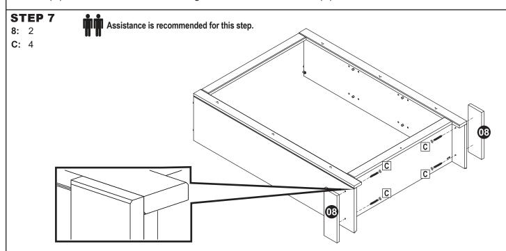
**NOTE:** Have an assistant firmly hold the trim boards in place to ensure they remain flush with the unit while hardware is secured.
