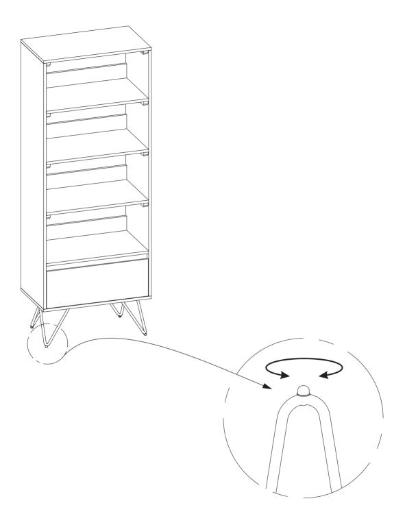
Note: Levelers on bottom of legs can be adjusted if floor is uneven.
