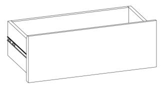
1. Place Drawer Frame  $\stackrel{\textstyle (E)}{\textstyle}$  on a flat, smooth surface and remove drawer by pressing clip.
