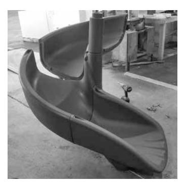
3. Attach the next curved section using 3/8"x3" stainless steel lags. Start with the bottom outside hole.(DO NOT OVERTIGHTEN!) Repeat this step until all curved sections are in place.
