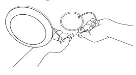
2a Align the friction clips to the housing and press the fixture flush to the ceiling.
