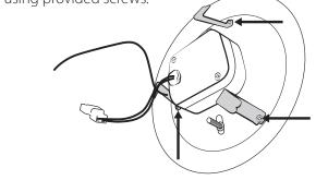
Disconnect Edison base from downlight and screw into socket inside recessed housing. (GU24 base option available). (Base not needed if using NICOR 19000A-LED-ID)
