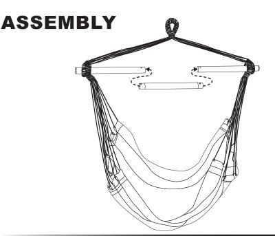
Align the spring button on Crossbar (B) with the hole in the spreader bar on Hammock Chair (A). Press the spring button down and carefully slide the crossbar into the spreader bar; the spring button will snap through the hole in the spreader bar when it is connected.
