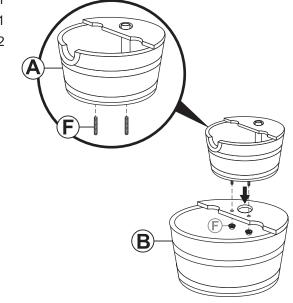
Install two Grub Screws (F) into the underside of Top Barrel (A). Place the top barrel onto Bottom Barrel (B) and secure using Nuts (F).
