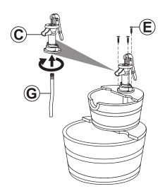
Firmly attach Water Tube (G) to Decorative Pump (C).
