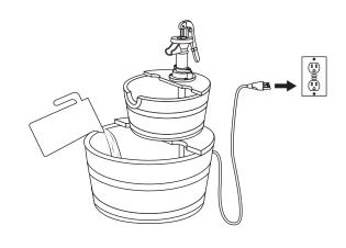
Fill each barrel with enough clean water to keep the pump fully submerged during operation, approximately 5.5 gallons (20.8L) total.
