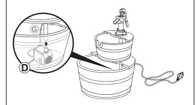
Place Electric Submersible Pump (D) in the bottom barrel. Run the power cord through the hole in the back of the barrel. Firmly connect the pump to the water tube.
