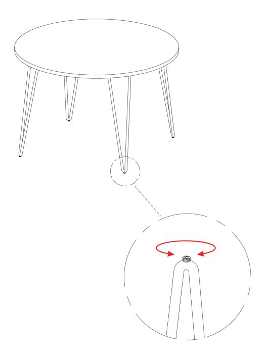
**Note:** Levelers on bottom of legs can be adjusted if floor is uneven.
