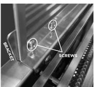
After installing the motor bracket, the motor will slide onto the bracket from the top with the cord pointing out and down and the motor output pointing in toward the center of the grill.
