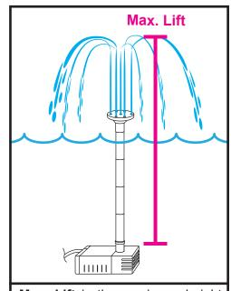
**Max.** Lift is the maximum height the pump will lift water.
