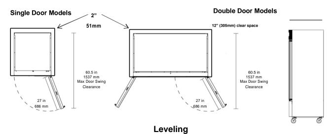
Ensure the floor where the unit is to be located is level. (It is ok to slope down from front to rear by up to 1/4" – it mustn't slope from the rear to the front.
