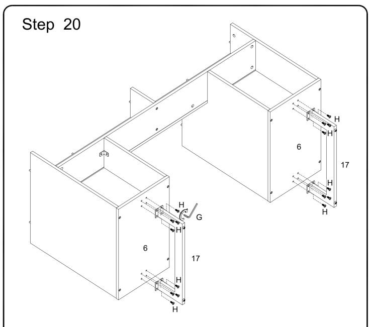
Using Bolt (H) attach part (17) to part (6) with Hex key (G) as per diagram.
