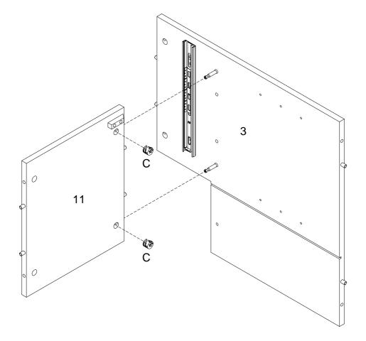
Using Cam lock (C) secure part (11) into part (3) with Philips head screwdriver as per diagram.
