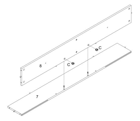
Using Cam lock (C) secure part (8) into part (7) with Philips head screwdriver as per diagram.
