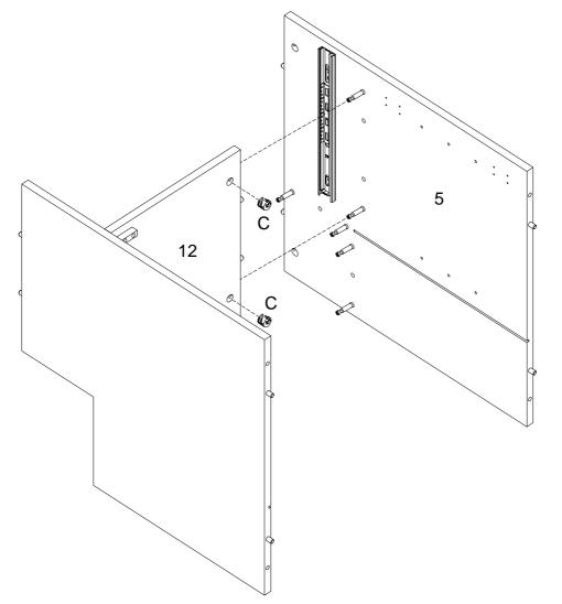
Using Cam lock (C) secure part (12) into part (5) with Philips head screwdriver as per diagram.
