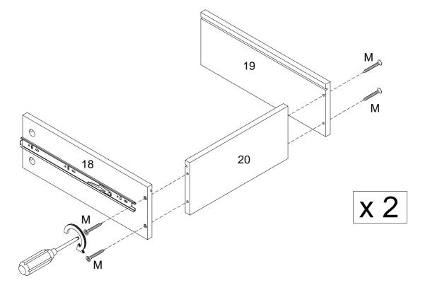
Using Screw (M) attach parts (18,19) to part (20) with Philips head screwdriver as per diagram.
