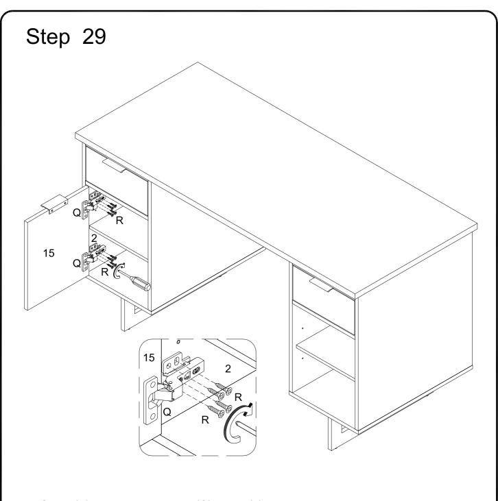
Using Screw (R) attach Europe Hinge (Q) to part (2) with Philips head screwdriver as per diagram.
