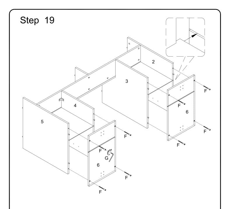
Using Screw (F) attach part (6) into parts (2,3,4,5) with Hex Key (G) as per diagram.
