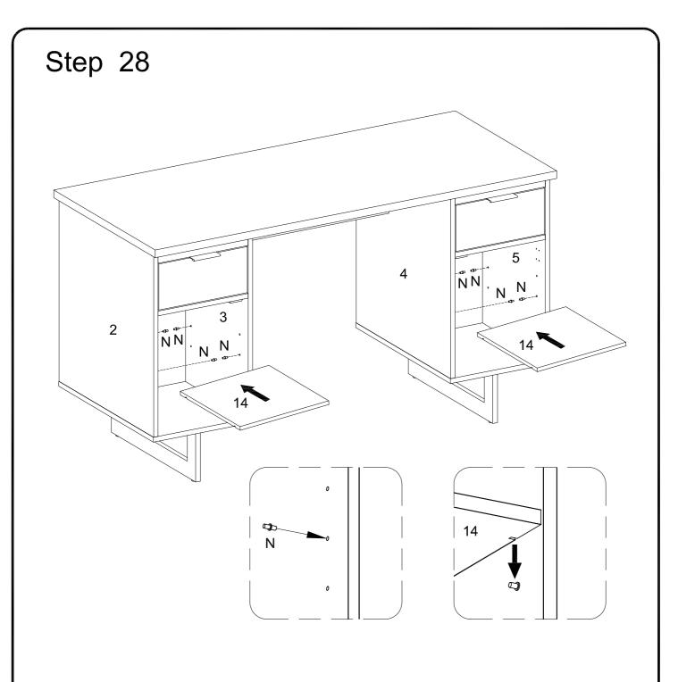
Insert shelf support pin (N) into parts (2,3,4,5) as per diagram. Make sure you place the shelf support pins (N) in the same level. So the shelf is not titled .Put part (14) into unit as per diagram. Tilt and rest the adjustable shelf (14) onto the shelf support pins .
