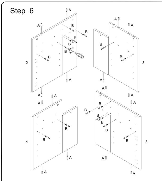
Insert wooden dowel (A) into parts (2,3,4,5) ,then secure Cam bolt (B) into parts (2,3,4,5) with Philips head screwdriver as per diagram.
