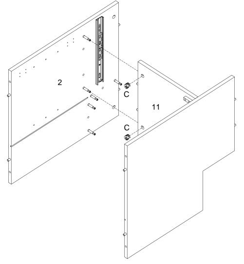
Using Cam lock (C) secure part (11) into part (2) with Philips head screwdriver as per diagram.
