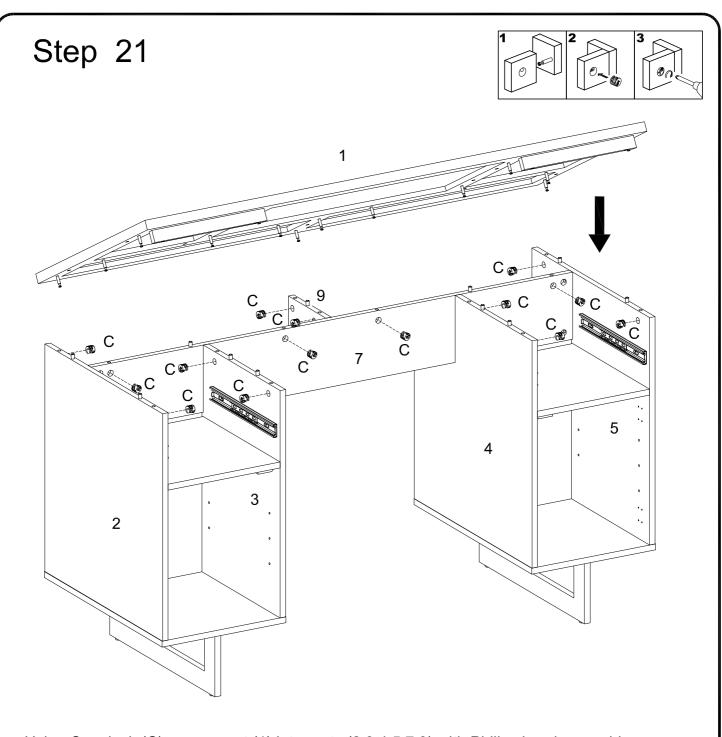
Using Cam lock (C) secure part (1) into parts (2,3,4,5,7,9) with Philips head screwdriver as per diagram.
