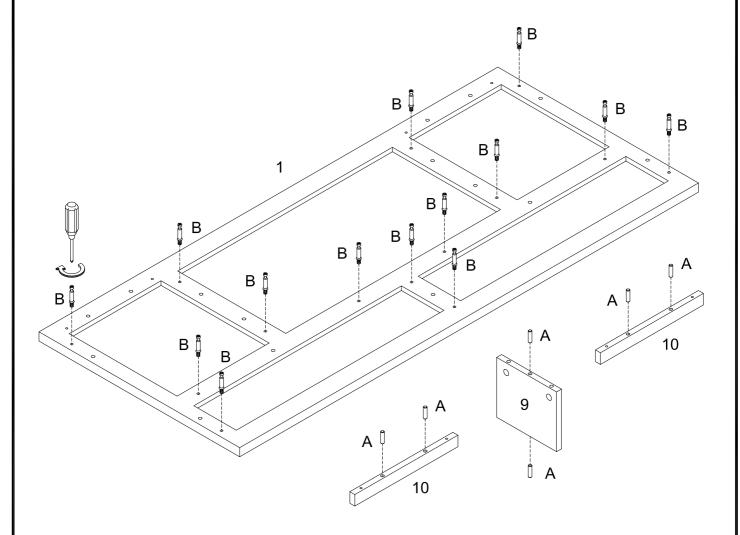
Insert wooden dowel (A) into parts (9,10) ,then secure Cam bolt (B) into part (1) with Philips head screwdriver as per diagram.
