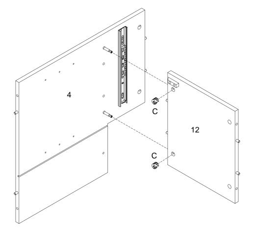
Using Cam lock (C) secure part (12) into part (4) with Philips head screwdriver as per diagram.
