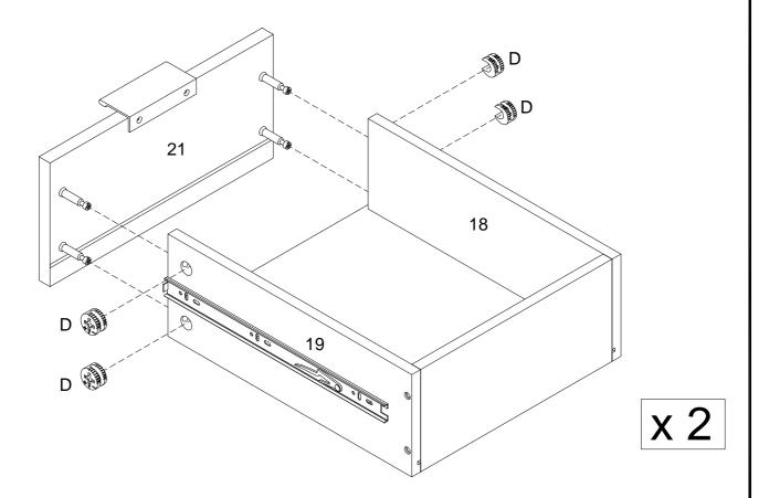
Using Cam lock(D) secure part (21) to parts (18,19) with Philips head screwdriver as per diagram.
