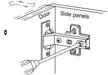
In-and-Out by loosening the hinge-arm mounting screw or via cam adjustment
