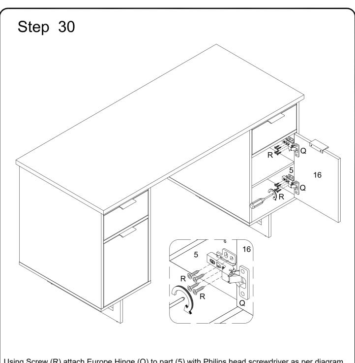
Using Screw (R) attach Europe Hinge (Q) to part (5) with Philips head screwdriver as per diagram.
