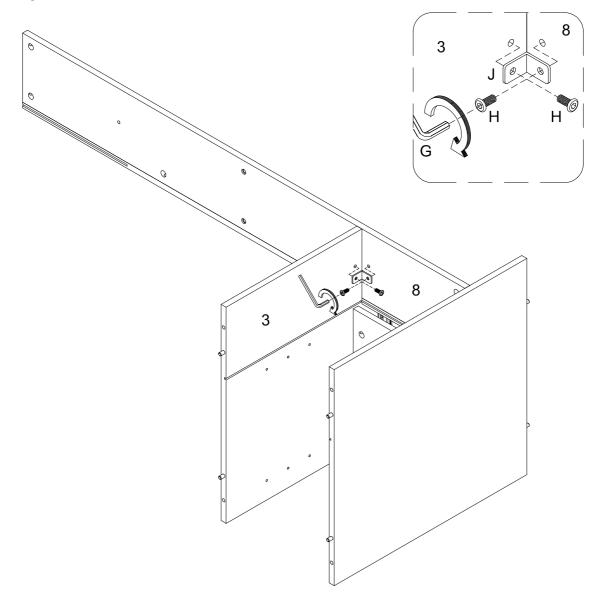
Using Bolt (H) attach Connecting Iron Sheet (J) to parts (3,8) with Hex Key (G) as per diagram.
