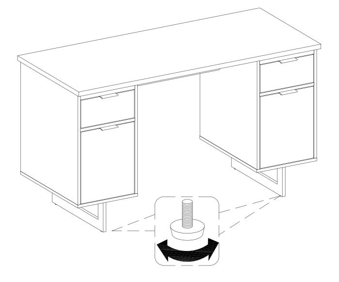
Position the assembled unit at the desired location ,if necessary adjust the floor leveler at the bottom of the leg to level the unit .
