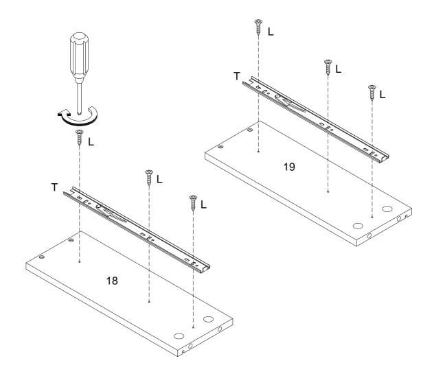
Using Screw (L) attach part (T) to parts (18,19) with Philips head screwdriver as per diagram.
