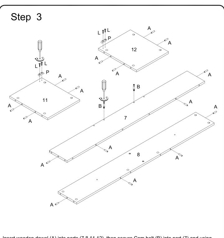
Insert wooden dowel (A) into parts (7,8,11,12) ,then secure Cam bolt (B) into part (7) and using Screw (L) attach door stopper (P) to parts (11,12) with Philips head screwdriver as per diagram.
