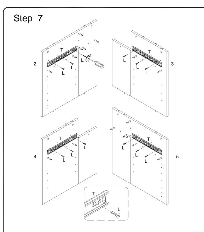
Using Screw (L) secure part (T) into parts (2,3,4,5) with Philips head screwdriver as per diagram.
