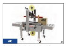
3M-Matic™ Adjustable Case Sealer a80 is an adjustable side belt drive case sealer that dependably seals uniform size cases.
