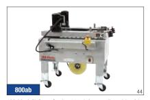
3M-Matic™ Case Sealer 800ab is an adjustable side belt drive case sealer. Applies bottom seal only at rates up to 40 cases per minute, using tape widths from 36mm to 48mm, and also 72mm tape.
