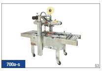
3M-Matic™ Adjustable Case Sealer 700a-s stainless steel has advanced features to seal uniform cases up to 30 per minute. Dual masts with dual lead screws for stability and uniform height adjustments. Adjustable top and bottom belt drive system for reliable conveyance of heavier or tall/light boxes. Compression rollers position each box for precise tape sealing. Stainless construction for corrosive environments.
