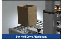
Holds RSCs on the optional infeed conveyor to free the operator's hands for case filling.
