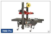
3M-Matic™ Random Case Sealer 7000r Pro is a semi-automatic random case sealer that automatically adjusts for case height and width and is capable of sealing 24 cases per minute, using tape widths from 36mm to 48mm wide.
