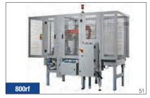
3M-Matic™ Case Sealer 800rf Type 40800 is a fully automatic random size case sealer that automatically adjusts for various case sizes and folds the top minor and major flaps up to 10 cases per minute. Using tape widths from 36mm to 48mm tape widths.
