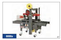
3M-Matic™ Side Belt Adjustable Case Sealer 8000a is an adjustable side belt drive case sealer. Seals up to 40 cases per minute, using tape widths from 36mm to 48mm, and also 72mm tape.
