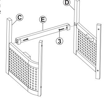
Loosely fasten Chair Support Bar (E) between Right Arm Panel (C) and Left Arm Panel (D) by handtightening two JCBC M6x40mm Bolts (3).
