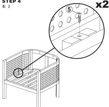
Fasten the top of the seat to the frame using two M6x30mm Screws (5), as shown.
