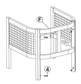
Loosely fasten Chair Back (F) to the arm panels by hand-tightening four JCBC M6x30mm Bolts (4).
