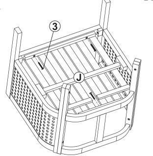
Fasten the underside of Chair Seat (J) to the chair frame using three JCBC M6x40mm Bolts (3).
