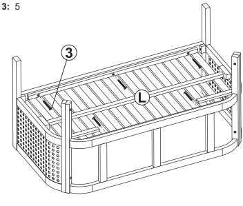
Fasten the underside of Loveseat Seat (L) to the loveseat frame using five JCBC M6x40mm Bolts (3). Finish tightening all bolts.
