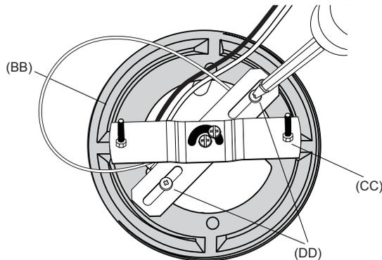
**4** Using the Wire Nuts (HH) provided, connect the white fixture wire to the neutral (white) supply wire. Connect the black fixture wire to the hot (black) supply wire. Connect the ground or bare supply wire to the ground screw of the crossbar.
